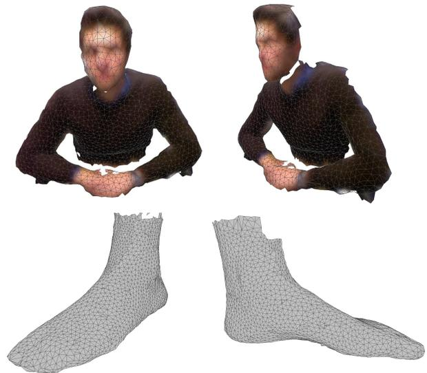
Fig. 10. Reconstruction of 3D human models with the proposed method. Top: 3D model of a person. Bottom: digitized human foot.
