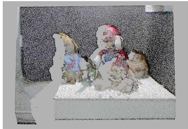
(b) Filtered point cloud using GNG + Color interpolation (50,000 points)
