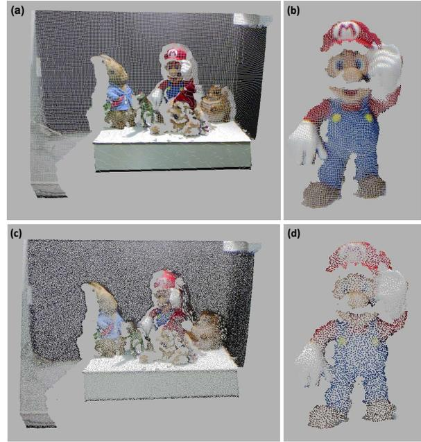
Fig. 1. Different objects are down-sampled using the Colour-GNG representation. (a),(b) show original pointclouds. (c),(d) show down-sampled point clouds using the proposed method.
