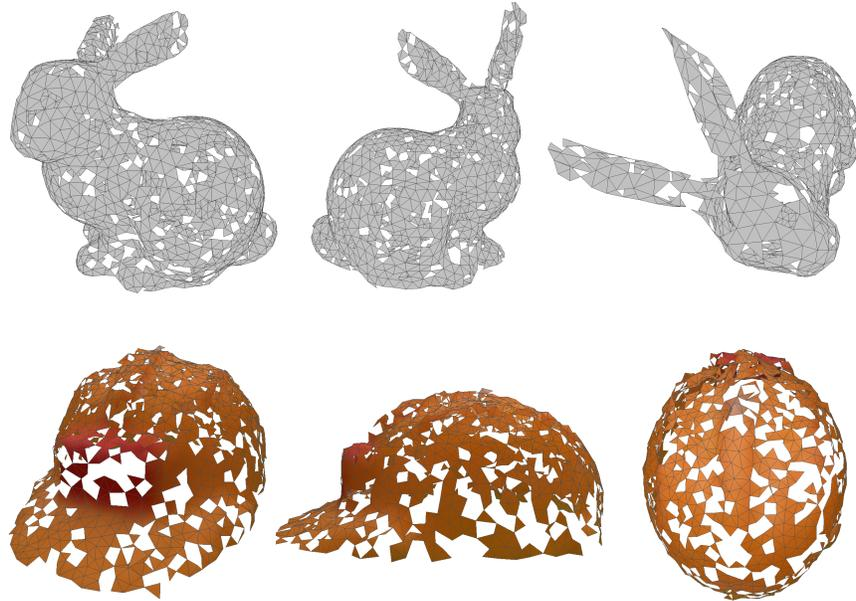
Fig. 5. Different views of reconstructed models using an existing GNG-based method for surface reconstruction. Post-processing steps were avoided causing gaps and holes in the final 3D reconstructed models.
