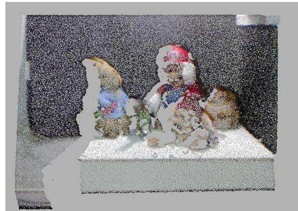
(c) Filtered point cloud using Color-GNG (50,000 points)
