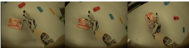
Fig. 5. An example of a series of images collected during a PUSH action with the *iCub* robot.
