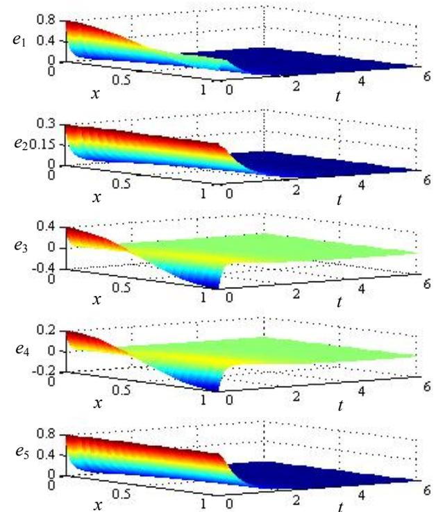
Fig. 2 Closed-loop error profiles of evolution of  $e_i(x, t)$ ,  $i \in \{1, 2, \dots, 5\}$
