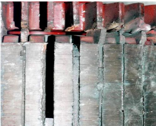
Fig. 7. The faulty cage with several cracked and broken rotor bars
