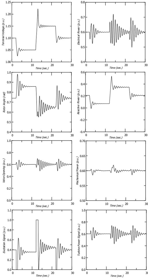
Fig. 2: Simulated system response for 5% step changes in the desired terminal voltage, ( $P_e=0.6$  p.u.).
