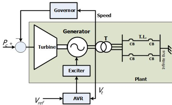
Fig. 1: A single-machine-infinite-bus with traditional control.
