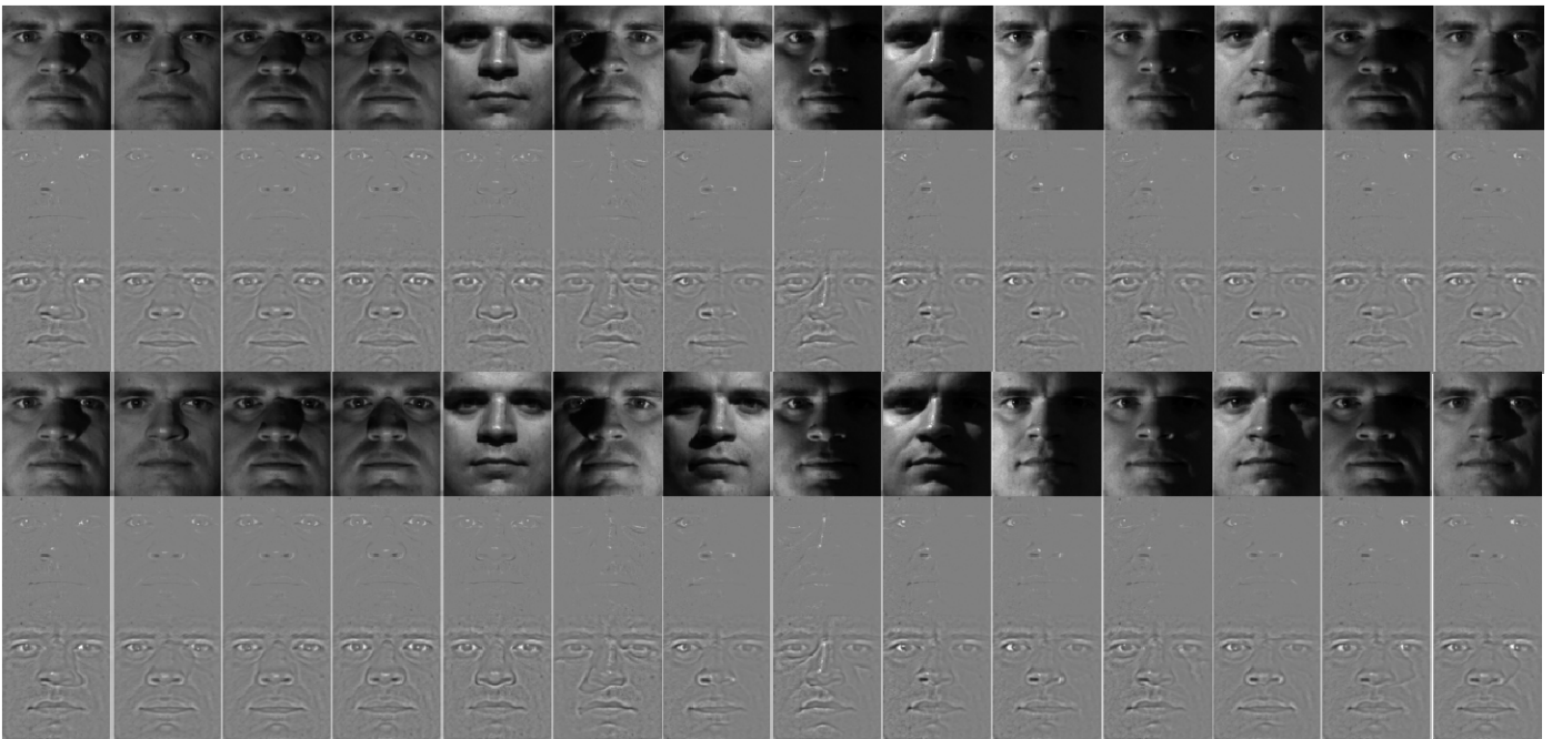
Fig. 5 Examples of illumination invariant feature extraction from the Extended Yale B Database. Three blocks represent three identities. Each identity shows face images under various illumination conditions. For each block, top row is the raw face images; middle row is the small scale using TV method; bottom row is the result using TV-NSCT method.
