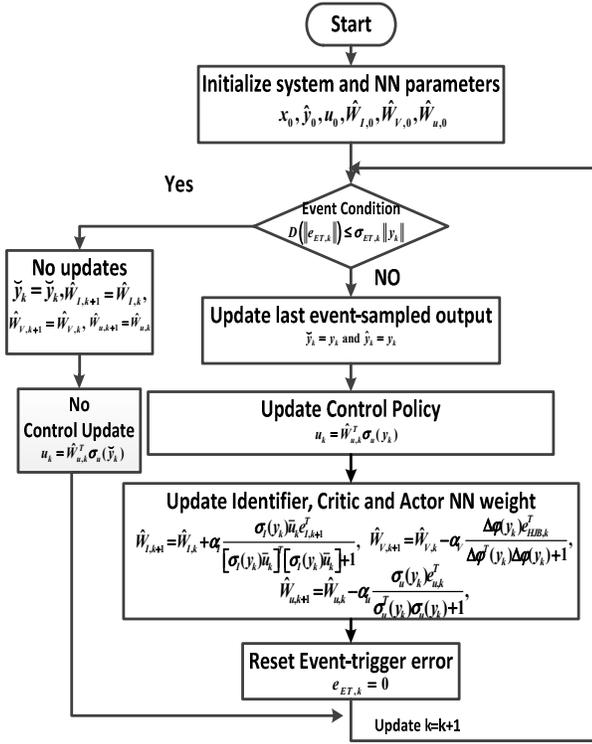
Fig. 2. Flowchart for the proposed event-triggered system
