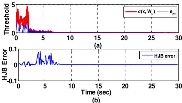
Fig. 4. (a) Triggering threshold with event-trigger error; (b) Temporal difference error.
