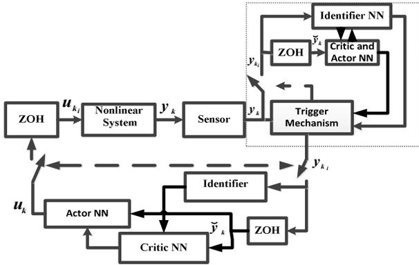
Fig. 1. Block diagram of an event-triggered near optimal control system.
