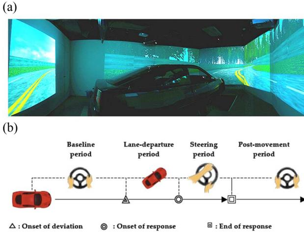
Fig. 1. (a) Three-dimensional-six-axis virtual reality (VR) scenario. (b) Schema for driving task in simulated scenario.
