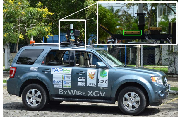
Fig. 3. Intelligent and Autonomous Robotic Automobile (IARA) with the mounted-on Point Grey Bumblebee XB3 camera (marked in green) used in experiments. Learn more about IARA at www.lcad.inf.ufes.br .
