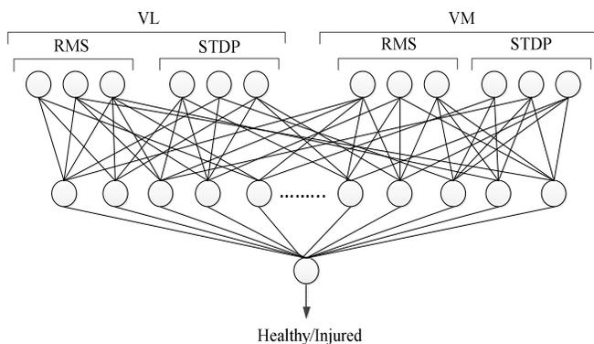
Fig. 9. ANN Architecture for Gait Patterns Identification using RMS and Soft Tissue Deformation Inputs of healthy/injured subjects.
