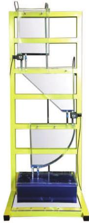
Fig. 3. Model of the Multi Tank system
