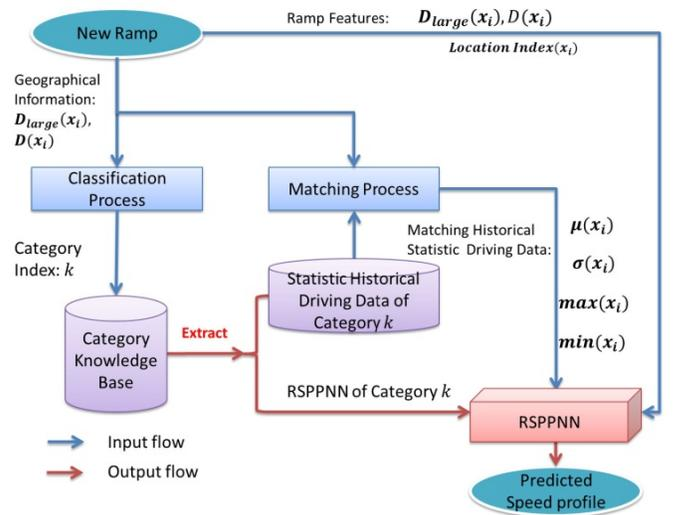
Fig.11. The architecture of an Intelligent Trip Modeling on Ramp (ITMR) System.
