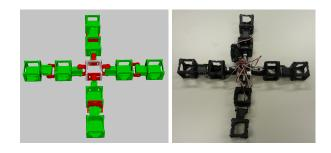
Figure 1: One of the RoboGen robots experimented with in this work. *Left:* In simulation. *Right:* In reality.
