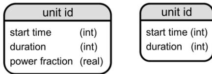
Figure 5: Structure of the proposed gene types for scheduling a generator unit with (left) and without (right) a unit-dependent power fraction parameter.
