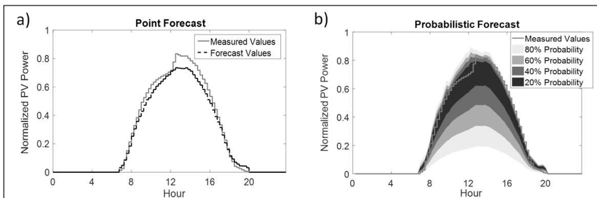
**Figure 2:** Examples of normalized PV power point and probabilistic forecasts: a: Point forecast; b: Probabilistic forecast: The intervals with lighter shades of gray encompass the darker intervals.
