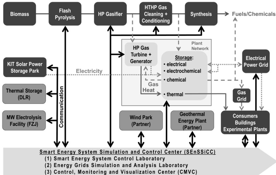
**Figure 1:** Energy Lab 2.0 components and connections [6]. Communication links are shown as solid black lines, while the energy and material flow is indicated by gray lines, which are solid, dotted, or dashed according to the transported medium. The figure shows existing facilities (dark gray), new components (light gray: SEnSSiCC, energy conversion and storage plant network), and external facilities (gray). Abbreviations: HP: High Pressure; HT: High Temperature.
