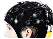
Figure 1: Enobio EEG cap used in this experiment. Source: neuroelectronics.com
