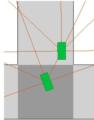
**Figure 1: Representation of two cars crossing a road intersection (darker area), equipped both with 5 radial proximity sensors. The sensors detect the distance to the roadsides, intersections, and other cars.**
