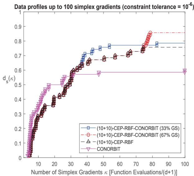
Figure 1: Data profiles for two variants of CEP-RBF-CONORBIT and for the component algorithms.
