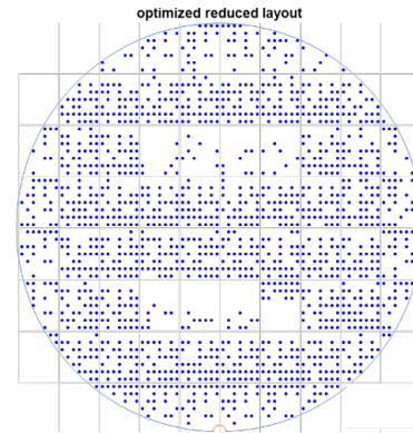
Figure 3: A reduced layout with 1591 marks (blue dots). Marks which are not read-out are not indicated.
