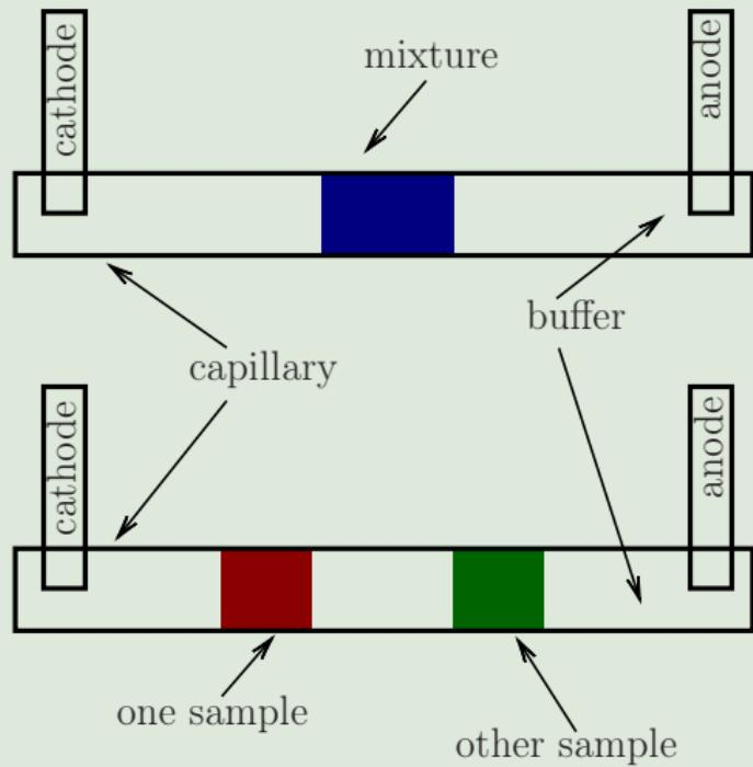
The interior of capillary is filled with an electrolyte. The sample to be analyzed is injected in the capillary. Due to electric field it travels down the capillary and forms some zones. So we have some travelling zones and we can identify a mixture.
