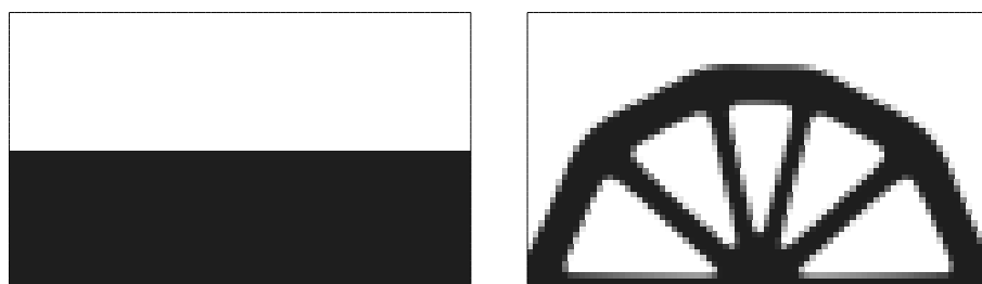
FIG. 2.4 – Optimal bridge in 2-d : iterations 6, 11, 16 and 100.
