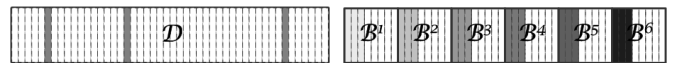
Fig. 1. Sparse signal models. Left: the overcomplete dictionary model. In this model any sparse set of atoms (columns in gray) can be selected. Right: the structured sparse model selection model. In this model, the dictionary is comprised of a family of orthogonal bases, only one selected at a time. The model selection is calculated with linear approximation in a best basis, i.e., only the first few atoms of one basis (in gray) can be selected.
